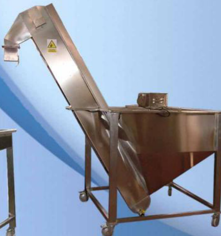
Loading hopper (Varios modelos) The product is immersed un water. It has a mixer for stir the potatoes
