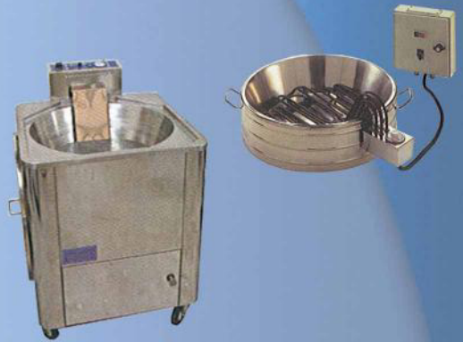
Electrical fryers Fryers with wheels made of stainless steel
