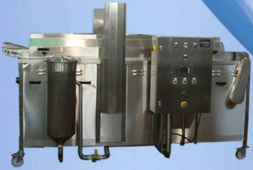
Nyt fryer and dispenser. Capacity 300k/h filters, pump... Several measures. custom manufacturing filters, oil levels, burners, multi-fuel, metal tapes ...
