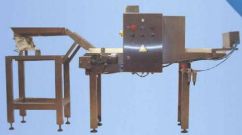
Black detector potatoes Removes the black potatoes that are fried.
