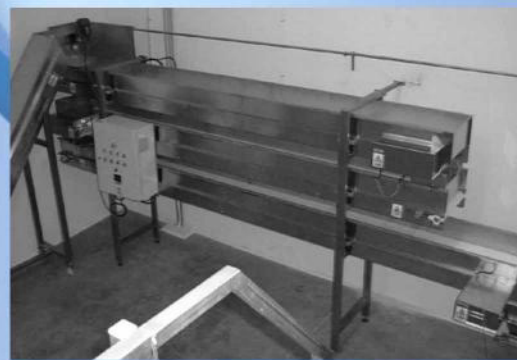
Cooler conveyor and accumaloyr Transports, accumulates, and cooled, the belt doesn't walk until the gap ins't completely filled.
