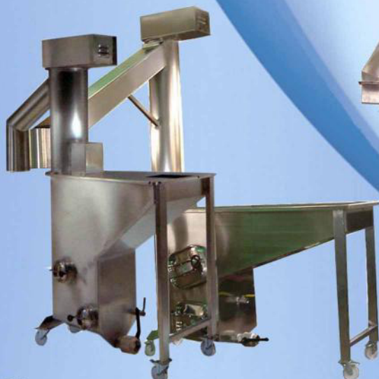
Stoner remover (2modelos) Through endless up potatoes and eliminate decantation stones and waste.
