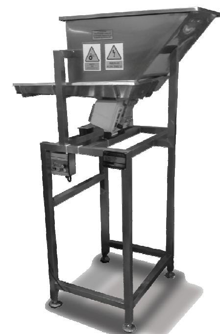
They incorporate a hopper that acts as an accumulator or lung. With a vibrating tray on the bottom where the product can move.
